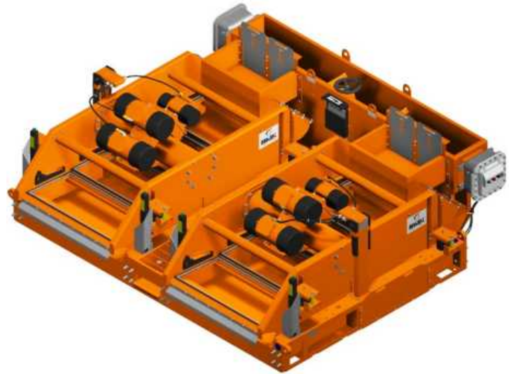
Figure 5 Dual Shaker with Common Possum Belly with Knife Gate
