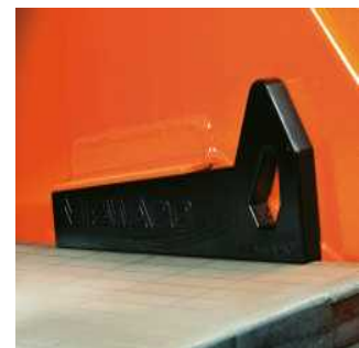
Figure 23 Wedge Positioned Between Screen Surface & Support Bar
