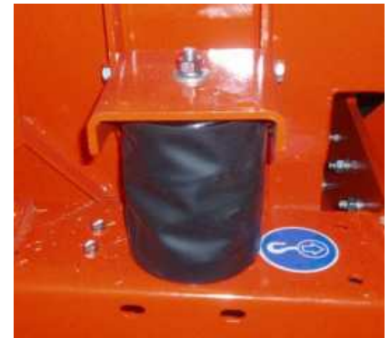
Figure 28 Spring Enclosed in Nitrile Boot
