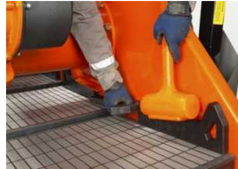
Figure 21 Meerkat Screen Removal
