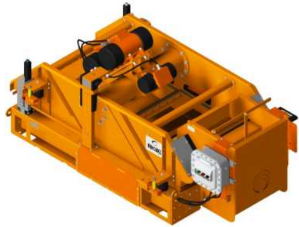
Figure 4 Possum Belly with Knife Gate Bypass
