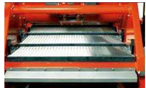
Figure 20 Screens & Wedges Firmly In Place
