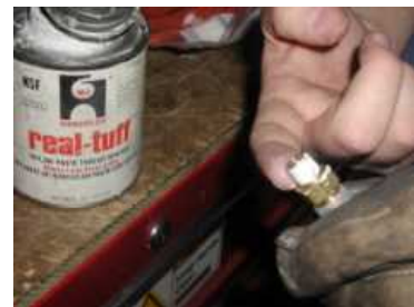
Figure 16 Sealant Used on Plug Threads
