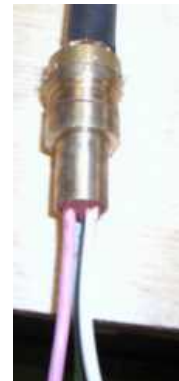
Figure 38 Compound Tube Filled with Epoxy Compound
