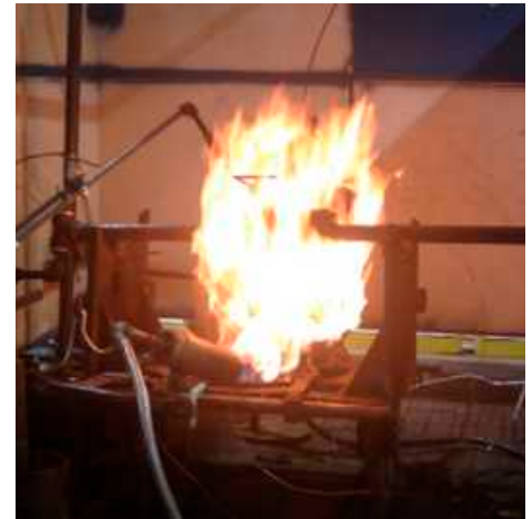
Fire test per API Spec 607 4th Edition.
