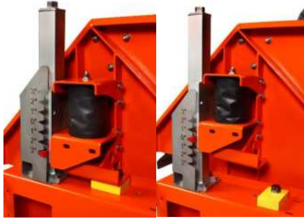
Figure 18. Discharge End Shipping Bracket Engaged (Left) and Stored (Right)
