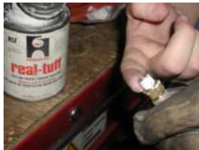
Figure 35. Sealant Applied on a Plug Thread
