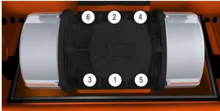
Figure 30. Motor Bolt Torque Pattern
