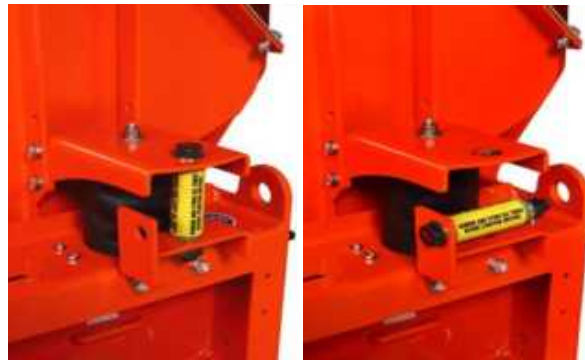
Figure 19. Feed End Shipping Bracket Engaged (Left) and Stored (Right)
