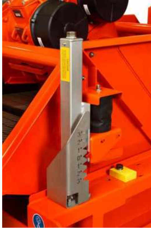
Figure 25. Basket (Deck) Elevator Jack
