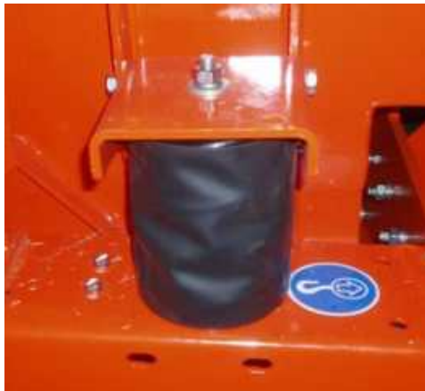
Figure 32. Spring Enclosed in Nitrile Boot
