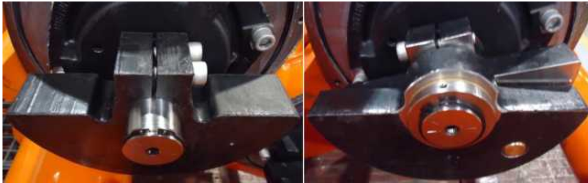
Figure 21. 60Hz Fixed Weight (Left) & Swing Weight (Right)
