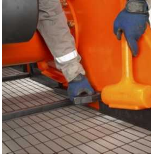
Figure 26. Use Extra Wedges with a Mallet to Loosen Screen Wedges
