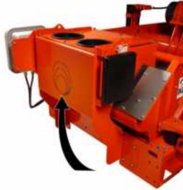
Figure 12. Piping Installation Guide Stenciling (Arrowed)
