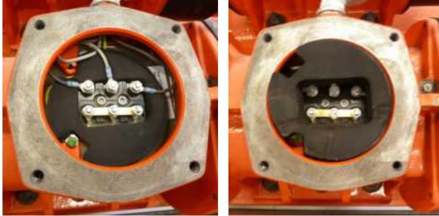
Figure 31. Thin Lower Isolator; Leads Showing (Left) and Thick Top Isolator; Leads Not Showing (Right)
