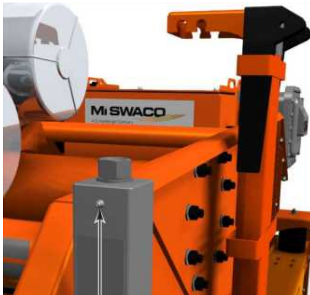
Figure 33. Grease Port on the Elevator Jack (Arrowed)
