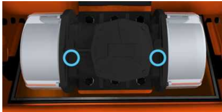
Figure 29. Grease Fittings (Circled)
